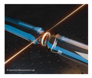
Light (shown in orange) is injected into an optical microresonator via a tapered optical fibre. The light circulates many thousands of times inside the structure and couples strongly to high-frequency acoustic waves.
